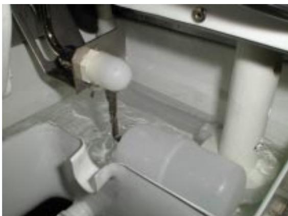
When the float has been risen from the water filling the Sump Assy, the water has forced all trapped air out of Water Pump and pump tube, thus preventing the pumping of water filled with air bubbles.
